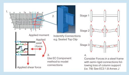
Figure 1. Wp1: East Penthouse Collapse Connections Analysis
