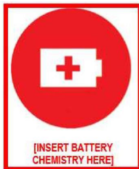
Figure 20: Battery Chemistry marking
