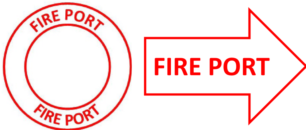
Figure 27: Fire Port marking
