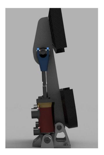
Using the end mounted master cylinders, especially with the trunnion mounts allows the balance bar to be on the pedal box not in the pedal: this makes fitting the bias adjuster cable a lot easier and makes the pedal design simpler.
